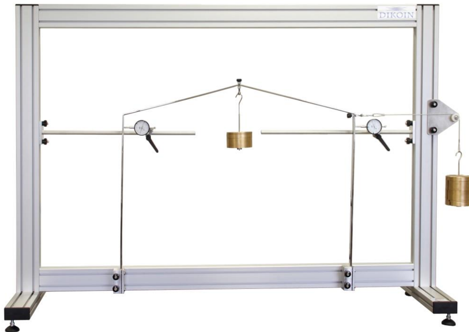
View of the assembled pitched-roof frame.
